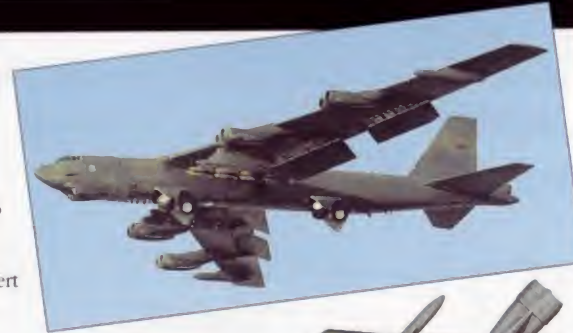
'Buffs' can mount up to 24 340-kg (750-lb) or 454-kg (1,000-lb) high-explosive or cluster bombs on external wing pylons.
